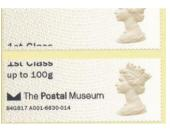
Two major errors occurred simultaneous on 7-Apr-17 - the guillotine to cut between the stamps appears to be set at 1½ and 1½ of a stamp repeating and the printer appears to be set at 1½ stamps. Resulting in a complete stamp only every third label.
